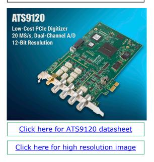
**ATS9120**<sup>®</sup> features two simultaneous analog input channels that can each be sampled at rates up to 20 MS/s with 12 bit vertical resolution. Each channel has 10 MHz of full power analog input bandwidth. With software selectable attenuation, users can achieve an input voltage range of  $\pm 40$  mV to  $\pm 20$  V. **ATS9120**<sup>®</sup> uses an on-board FIFO to temporarily store ADC data before DMAing it to motherboard memory.
